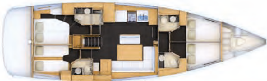
4 cabins version: Two transformable cabins forward, VIP aft cabin, aft guest cabin (optional saloon bench)
