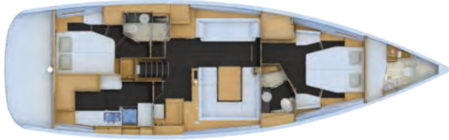
2 cabins version: Forward owner's cabin, VIP aft cabin, full saloon and aft galley (shown with optional skipper cabin)
