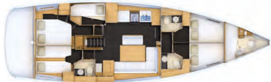
5 cabins version: Two transformable cabins forward, VIP aft cabin, aft guest cabin, lateral bunk cabin (optional saloon bench and skipper cabin)
