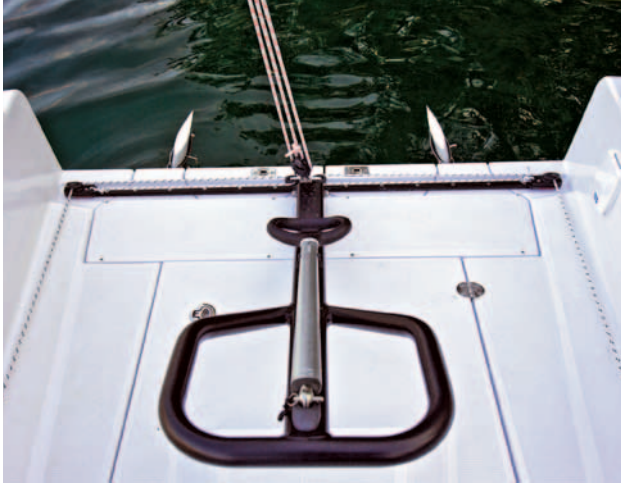
Single tiller for easy handling and maximum control. Mainsheet traveller mounted on the transom for maximum cockpit space (optional on S1).
