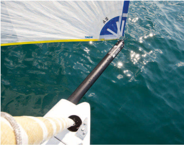
The retractable bowsprit brings an efficient asymmetric setting, bringing the rig's point of effort forward to enhance control at high speed.
