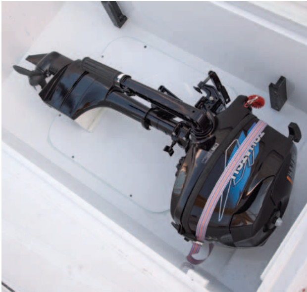
In the cockpit sole there is a designated locker for an outboard engine which can be deployed within a self contained cartridge system.
